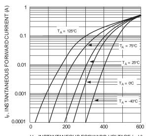
V<sub>F</sub>, INSTANTANEOUS FORWARD VOLTAGE (mV) Fig. 1 Typical Forward Characteristics
