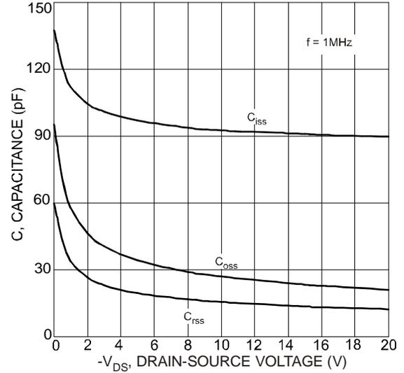
Fig. 10 Typical Capacitance
