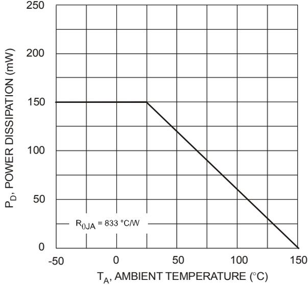
Fig. 1 Derating Curve
