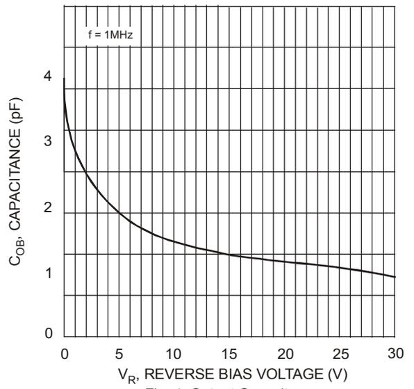
Fig. 4 Output Capacitance
