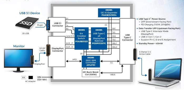
USB Type-C-LINK Monitor (CLM) Evaluation Board (EVB) System Configuration
