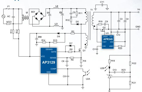
The APR349 is a secondary-side synchronous-rectification MOSFET driver optimized to co-work with the AP3129 for higher efficiency.
