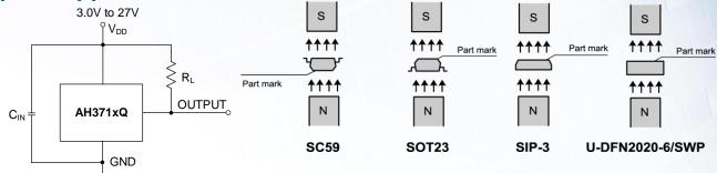
Note:  $C_{IN}$  is for power stabilization. To strengthen the noise immunity, the recommended capacitance is 10nF ~ 100nF.  $R_L$  is the pull-up resistor.
