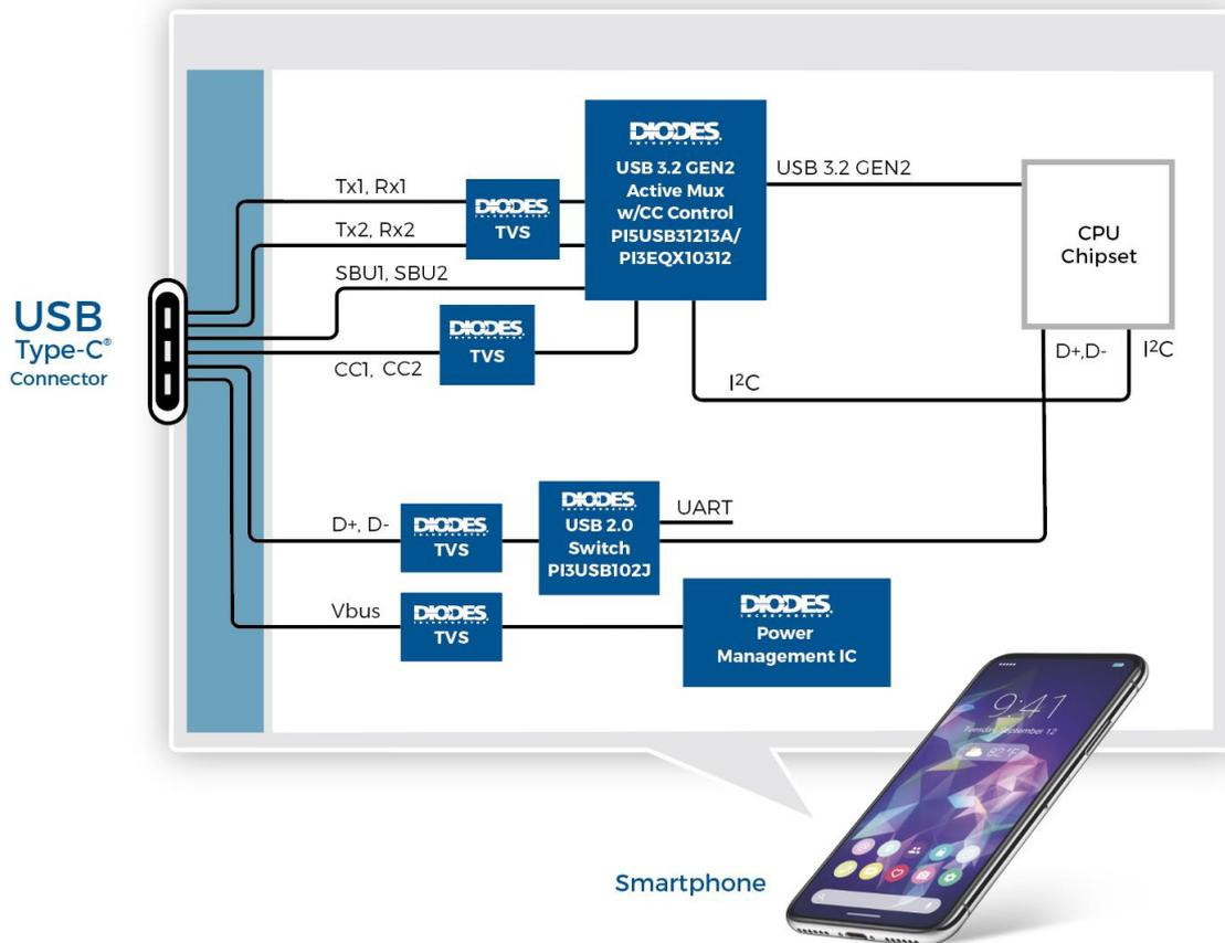
Figure 3. Highly Integrated and Protected USB-C Interface for Smartphones.
