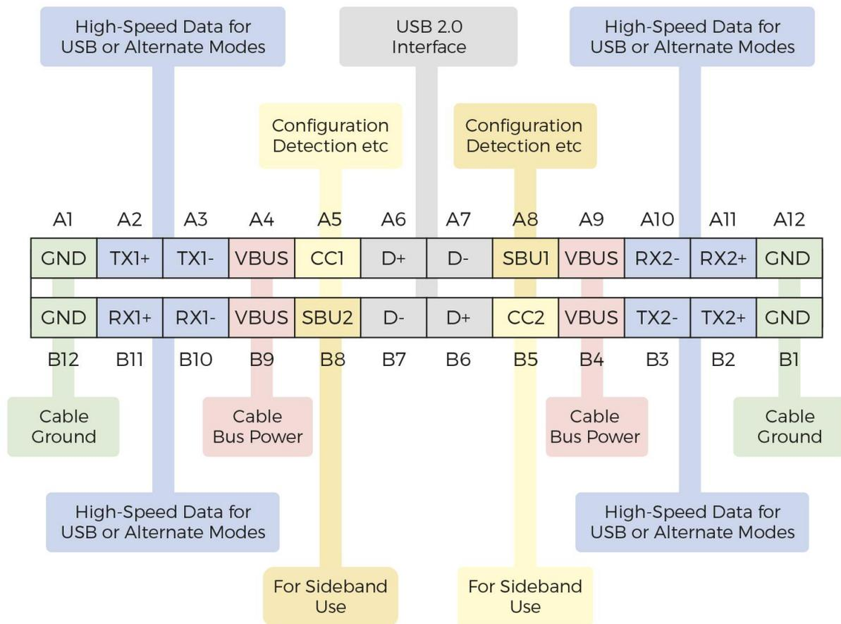
Figure 1. Pin Assignments in the USB-C Connector
