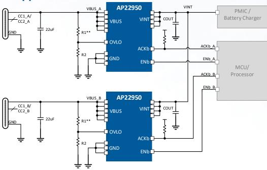
Overvoltage-Protected USB-PD VBUS Power Switches
