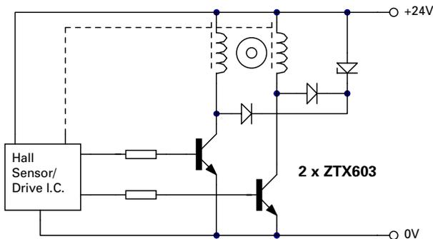
High power brushless fans incorporate Hall effect rotor sensors which directly control stator winding driver transistors. Since these drivers must withstand high surge and continuous currents which occur in normal and stalled operation, expensive TO220 or TO126 Darlington transistors are commonly specified.
