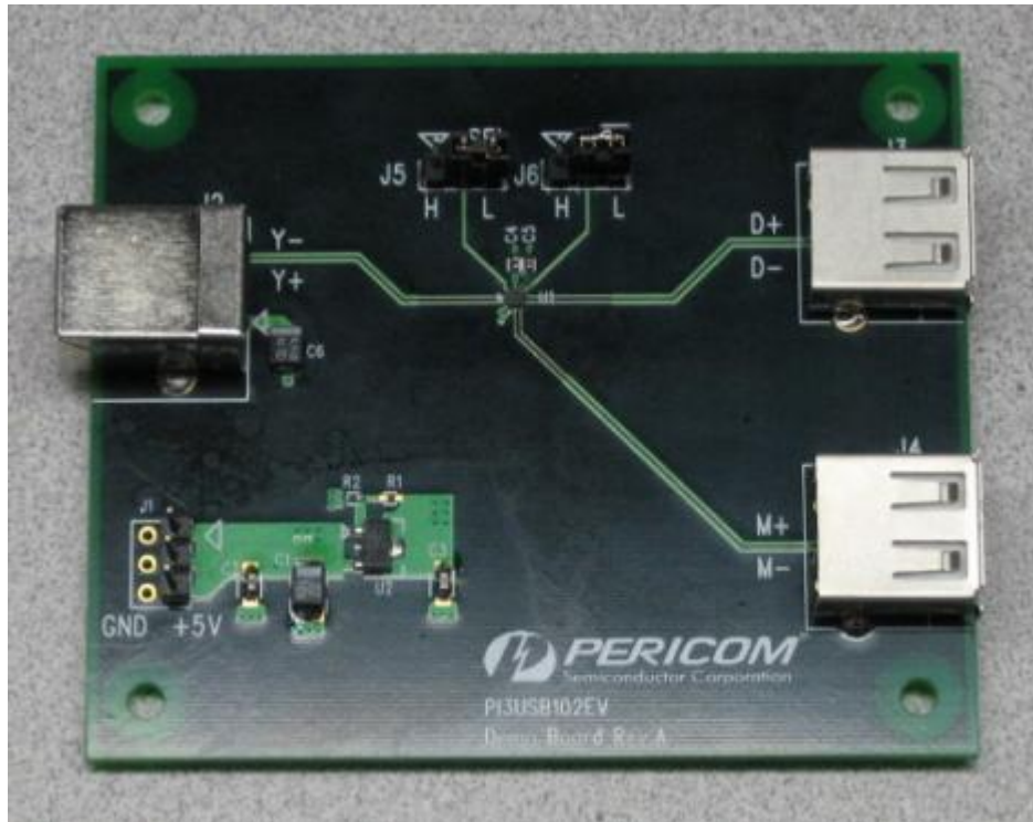
Figure 1. Top view of PI3USB102
