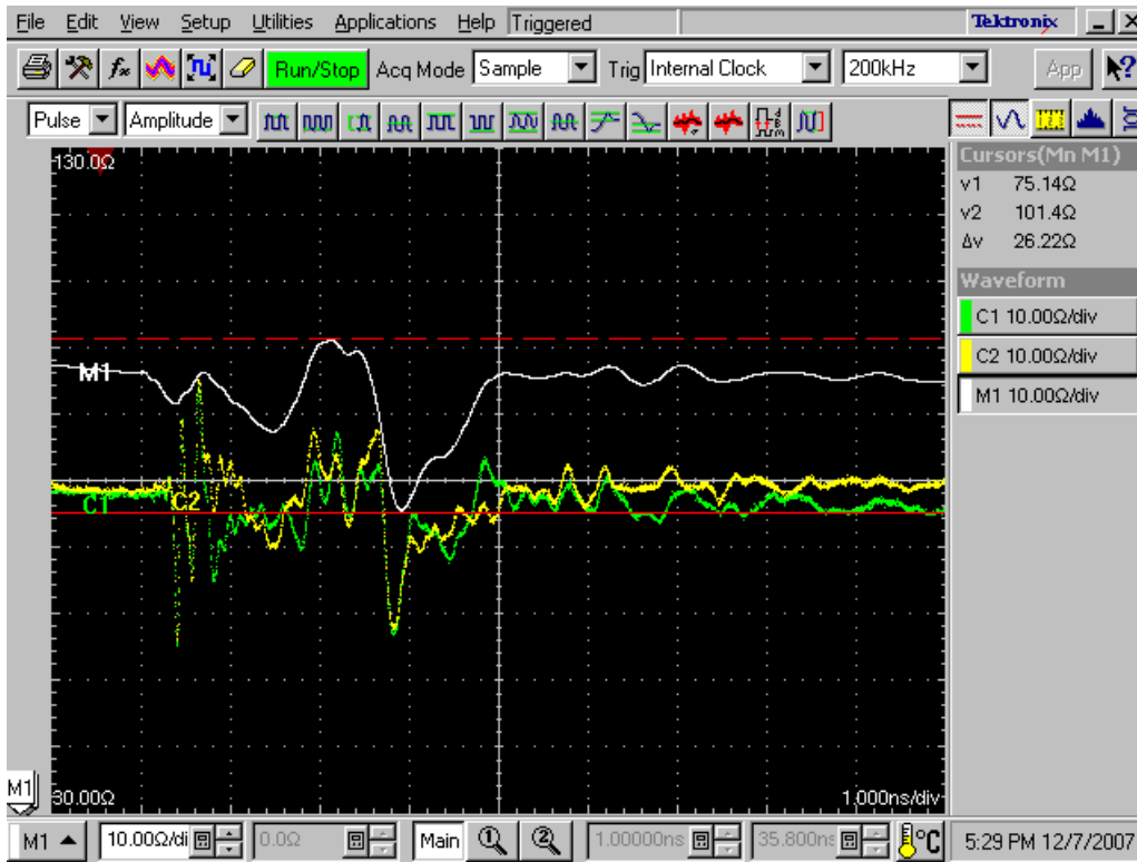
Figure 10b. TDR at D+/D- of J4
