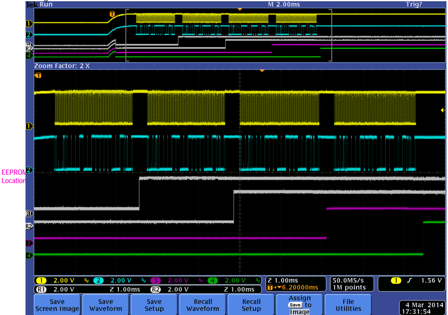
Figure4 Reading Waveform for Multiple ReDriver Application at I2C master mode
