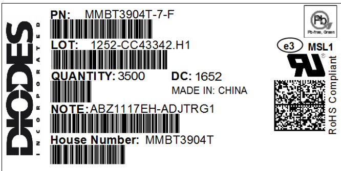
Fig. 4 Standard Label for a UL recognized, “Green” product, totally Lead-Free & fully RoHS Compliant with Tin terminal finish and Moisture Sensitivity Level 1.
