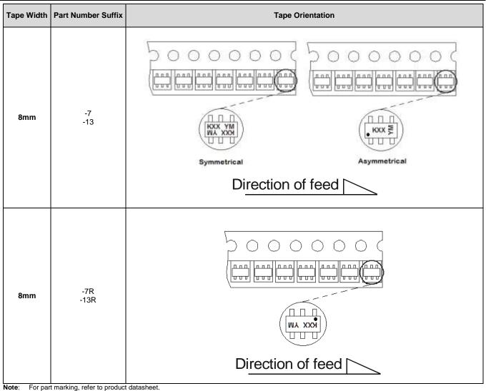
**Note:** Tape and package drawings are not to scale and are shown for device tape orientation only.
