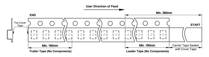
Note: There shall be a leader of at least 230mm which may consist of carrier tape and/or cover tape or a start tape followed by at least 160mm of empty carrier tape sealed with cover tape.
