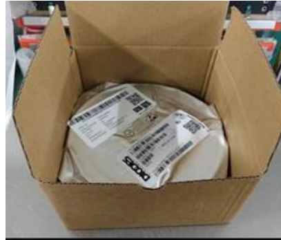
4.6: Opened inner box - vacuum sealed bag bag with MSL3 packing
