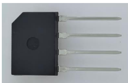
5.34: Through-hole sample before solder dip
