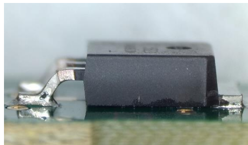
5.41: Sample after soldering on PCB
