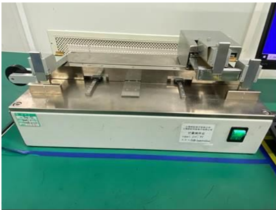
4.9: Peeling force measurement test setup
