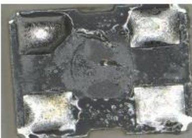
5.46: 2.0*1.6(mm) CXO SMD sample after soldering
