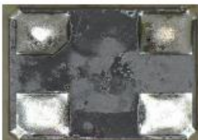
5.47: 3.2*2.5(mm) X-tal SMD sample after soldering
