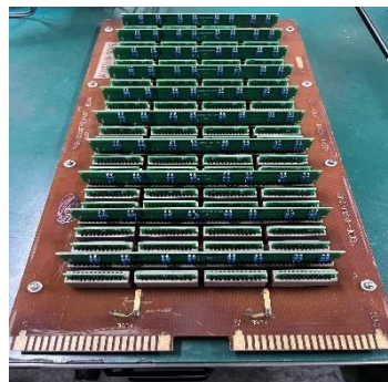
5.17: Small PCB on HAST Board
