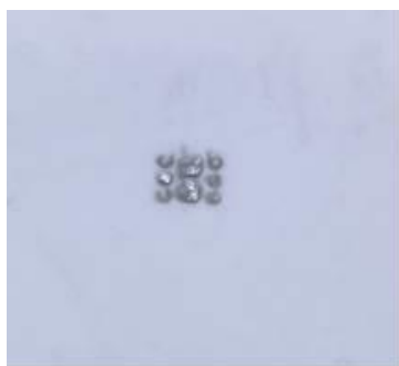
5.36: Solder printed by Stencil on ceramic board
