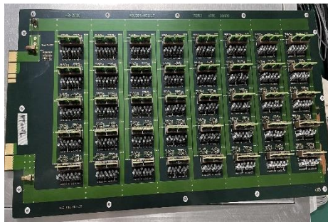
5.9: Small PCB on HTOL Board
