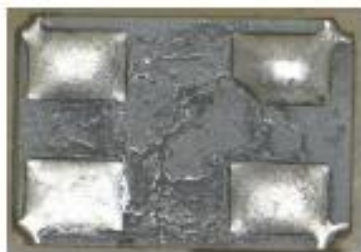
5.48: 1.6*1.2(mm) X-tal SMD sample after soldering
