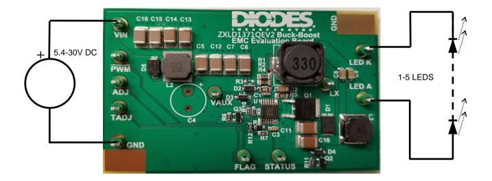
Figure 1: ZXLD1371QEV2 evaluation board and connection diagram
