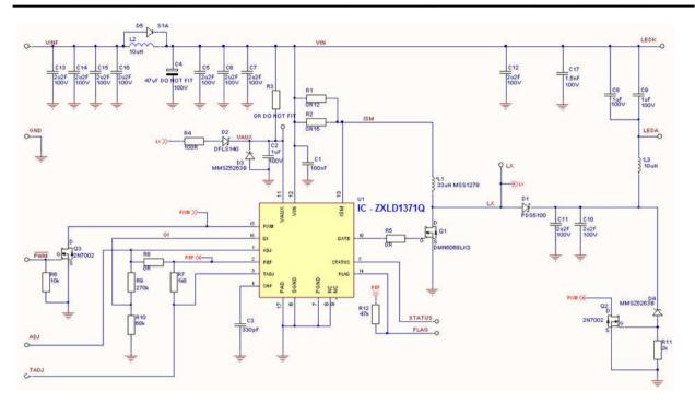
Figure 2: ZXLD1371QEV2 evaluation board Schematic
