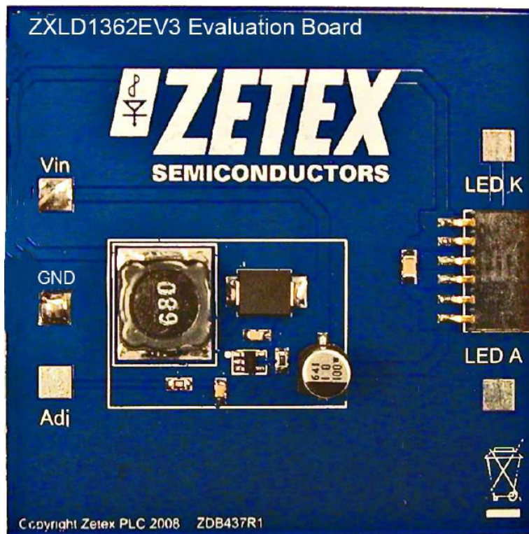
Figure 1 ZXLD1362EV3 Evaluation Board
