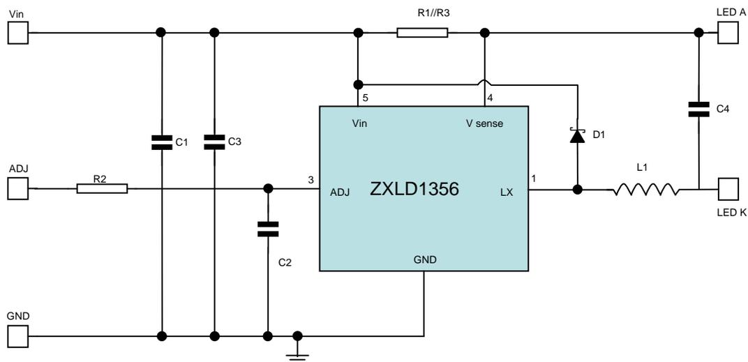
Figure 2: Schematic for the evaluation board ZXLD1356EV1
