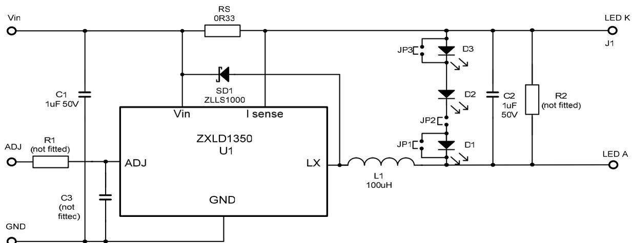
Figure 2: Schematic for the evaluation board ZXLD1350EV3
