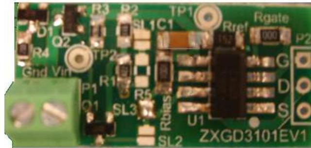
Figure 1 Evaluation board layout and connection diagram
