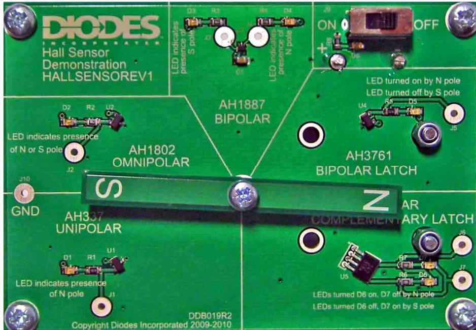
Figure 1: HALLSENSOREV1 Demonstration board
