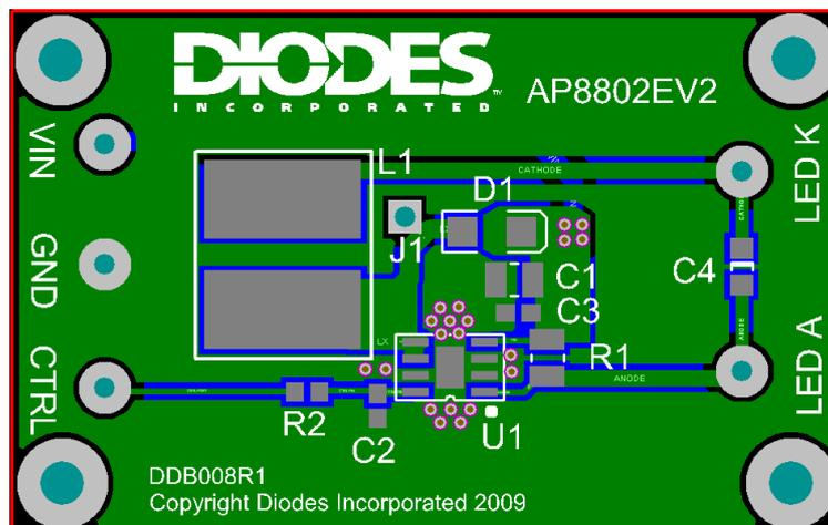
Figure 3: Component layout and circuit board view
