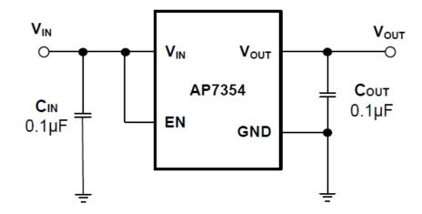
X5R- and X7R-type capacitors are suggested due to their minimal variation in value and ESR over temperature.
