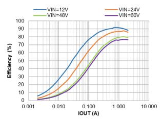
Figure 10. PWM Efficiency vs. IOUT, VOUT=3.3V, L=8.2 $\mu$ H
