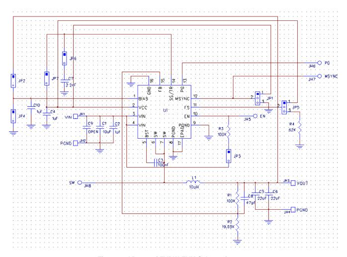
Figure 2. AP66200QFVBW-EVM Schematic
