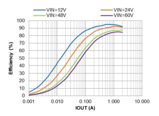
Figure 8. PWM Efficiency vs. IOUT, VOUT=5V, L=10µH
