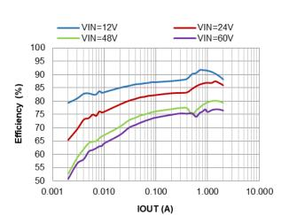
Figure 9. PFM Efficiency vs. IOUT, VOUT=3.3V, L=8.2µH
