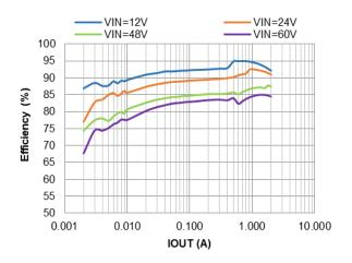
Figure 7. PFM Efficiency vs. IOUT, VOUT=5V, L=10µH
