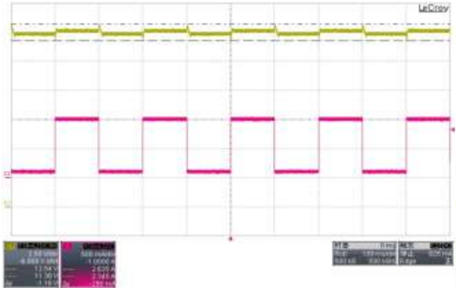
Figure 19: 90VAC; Load level: 0.1~1A; Vout: 12.58~11.38V
