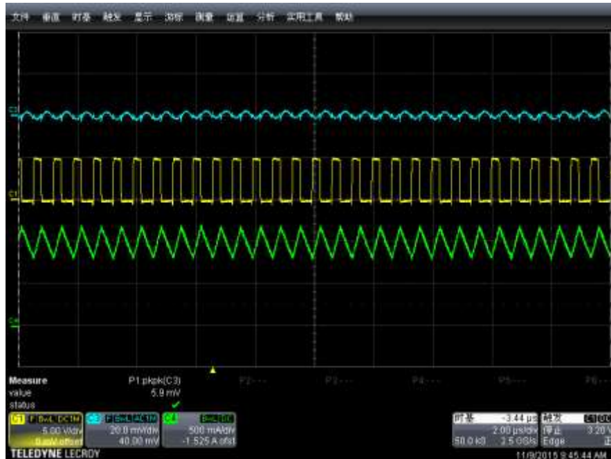
Operation waveform at Iout=1A (Blue-VoutAC; Yellow-Vsw; Green-IL)
