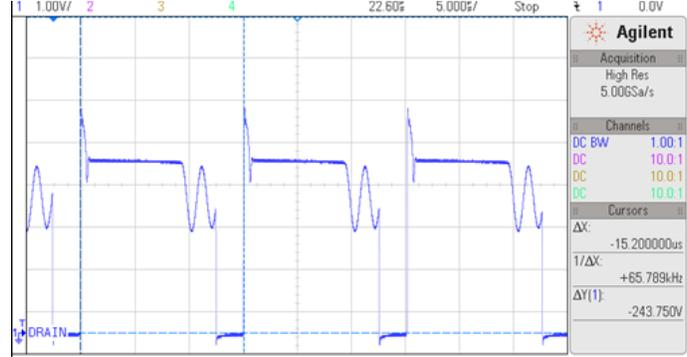
**Fig:7 Vds at full load by using DF probe 1:100 at 230V<sub>AC</sub>**
