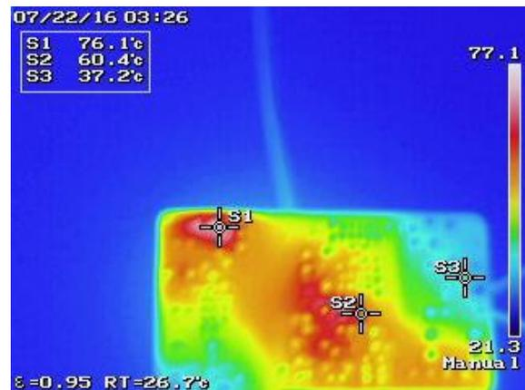
Figure:19 SMD side  $V_{in}=115V_{AC}$ , Test time=1hour
