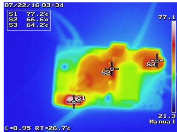
Figure:21  $V_{in}=115V_{AC}$ , Testing time = 1.15 hour
