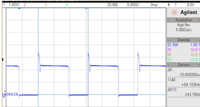
**Fig:6 Vds at full load by using DF probe 1:100 at 115V<sub>AC</sub>**
