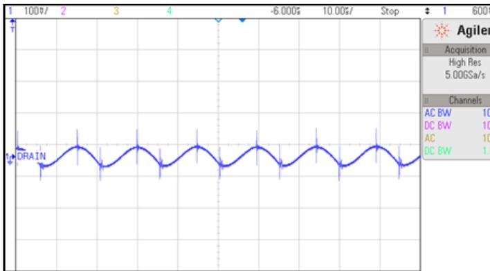
Figure:14 12V Ripple at 115Vac at FL .
