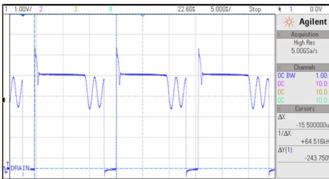
**Fig:8 Vds at full load using DF probe 1:100 at 265V<sub>AC</sub>**
