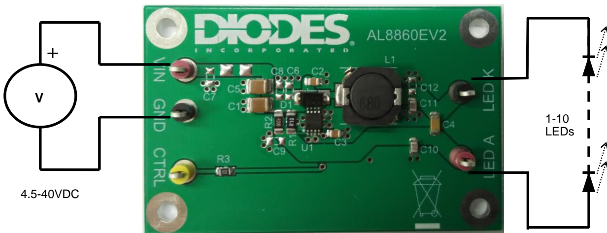
Figure 1: AL8860EV2 evaluation board and connection diagram
