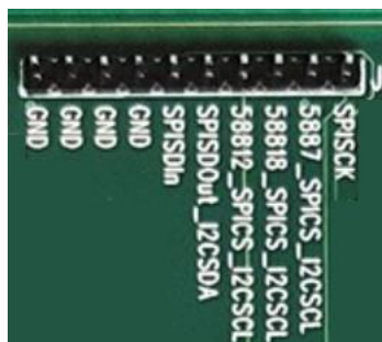
Figure 3: Box #5 - External I2C/SPI Connector Pinout
