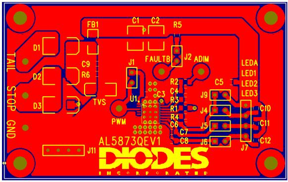
Figure 4. PCB Layout Top Layer View
