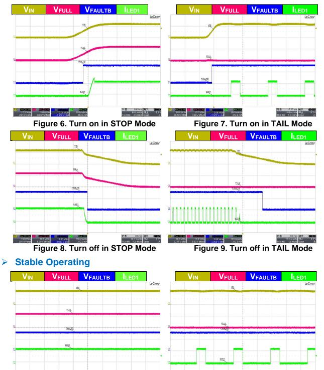
Figure 10. Stable waveform in STOP Mode Figure 11. Stable waveform in TAIL Mode
