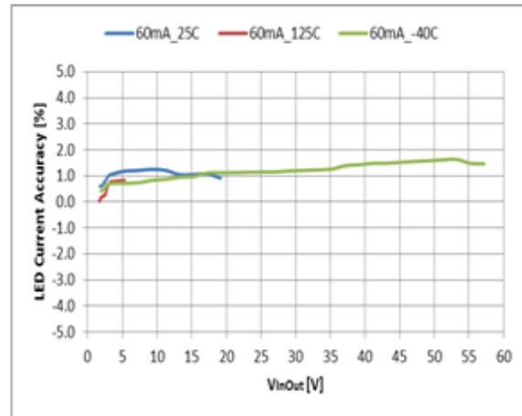
Figure 10 LED Current Accuracy (%) vs. VinOut across Temp
