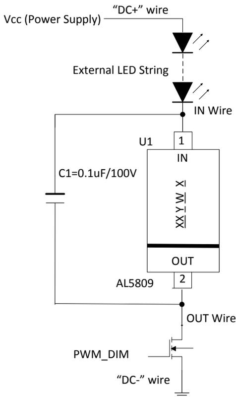
(a) PWM Dimming by External MOSFET
