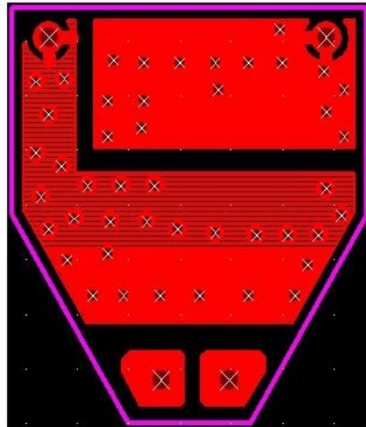
Note: This evaluation board provides design flexibility, multiple application circuits can be derived in both Low and High Side Current LED configurations. The footprint of U1 is compatible to both of **PDI-123** and **SOD-123** packages. In addition, it can be hooked up with use of PWM dimming.
