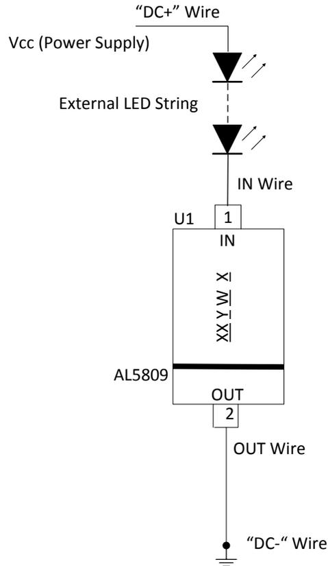
1. Depends on the current options, the evaluation board is as low side current LED configuration.
