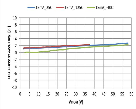
Figure 4 LED Current Accuracy (%) vs. VInOut across Temp
