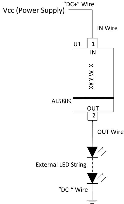
1. The evaluation can also be configured as High side current LED configuration.
