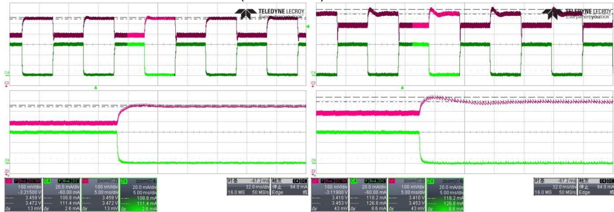
Figure 9: Load transient waveform with 120Vac (Left) and 230Vac (Right)
