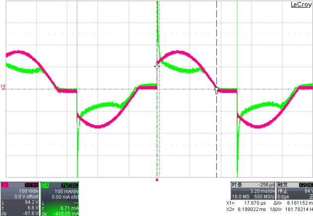
Input AC Current vs Dimmer Phase ( V_{in}=120V_{AC}/60Hz , Conduction angle 45deg)
