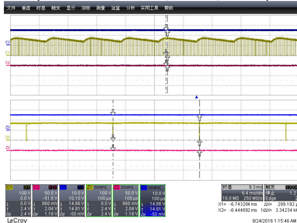
LED Short Protection (Vin=120V AC , Y-V DRAIN , R-V out , B-V CC )
