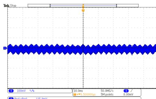
Figure 48: 90V<sub>AC</sub>/60Hz @20V/7A,  $\Delta V=115.9\text{mV}$
