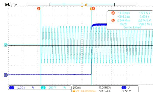
Figure 18: Start-up Time: 344ms at 3A Load
