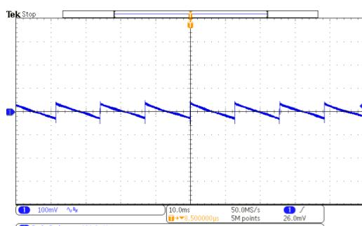
Figure 37: 264V<sub>AC</sub>/50Hz @5V/0A,  $\Delta V=101.0\text{mV}$
