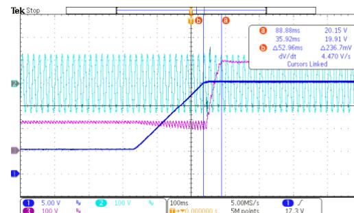
CH1:VBUS, CH2:AC Input, CH3:VPFC
