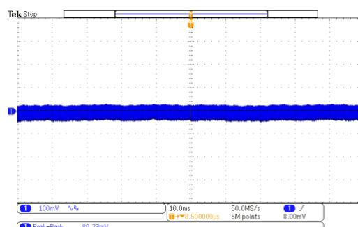
Figure 46: 264V<sub>AC</sub>/50Hz @15V/3A,  $\Delta V=80.23\text{mV}$
