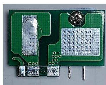
Figure 9: 140W ACF+GaN PD3.0 Adapter EVB DB1 PCB Layout
