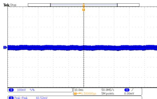
Figure 44: 90V<sub>AC</sub>/60Hz @15V/3A,  $\Delta V=60.52\text{mV}$
