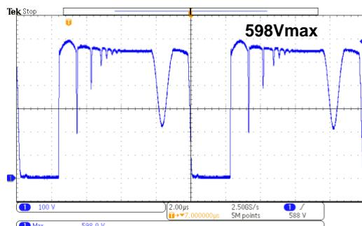
Figure 29: 20V/7A @90V<sub>AC</sub>/60Hz
