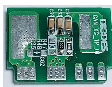
Figure 10: 140W ACF+GaN PD3.0 Adapter EVB DB2 PCB Layout
