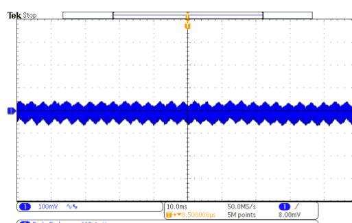
Figure 50: 264V<sub>AC</sub>/50Hz @20V/7A,  $\Delta V=112.1\text{mV}$
