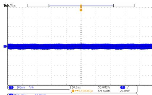
Figure 40: 90V<sub>AC</sub>/60Hz @9V/3A,  $\Delta V=67.86\text{mV}$
