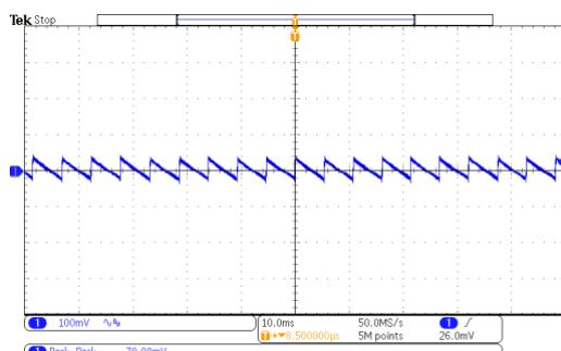
Figure 39: 90V<sub>AC</sub>/60Hz @9V/0A,  $\Delta V=78.88\text{mV}$
