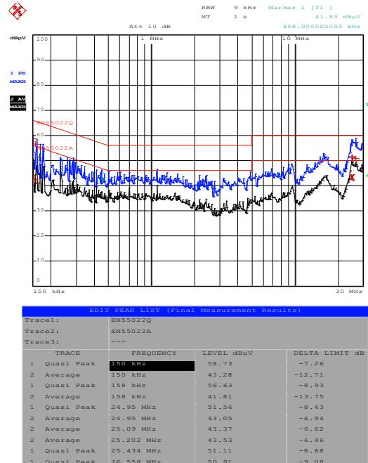
Figure 69: 115V<sub>AC</sub>/60Hz N line
