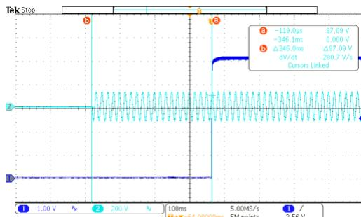
Figure 17: Start-up Time: 346ms at 3A Load
