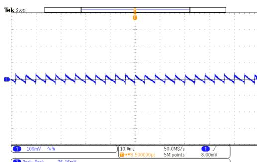
Figure 45: 264V<sub>AC</sub>/50Hz @15V/0A,  $\Delta V=76.16\text{mV}$
