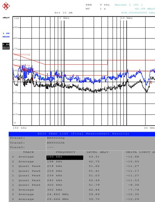
Figure 70: 230V<sub>AC</sub>/50Hz L line
