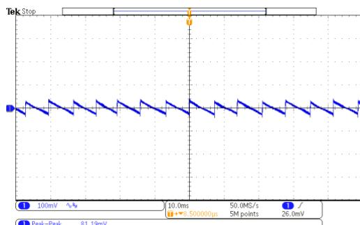
Figure 35: 90V<sub>AC</sub>/60Hz @5V/0A,  $\Delta V=81.19\text{mV}$
