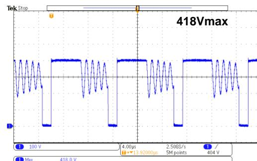
Figure 28: 20V/7A @264V<sub>AC</sub>/50Hz
