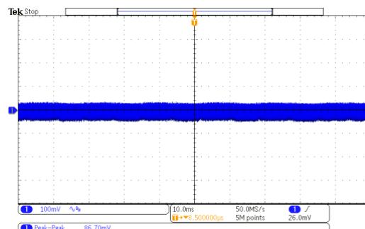
Figure 36: 90V<sub>AC</sub>/60Hz @5V/3A,  $\Delta V=86.70\text{mV}$
