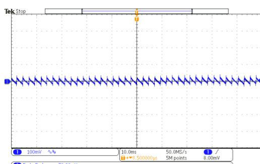
Figure 49: 264V<sub>AC</sub>/50Hz @20V/0A,  $\Delta V=70.09\text{mV}$
