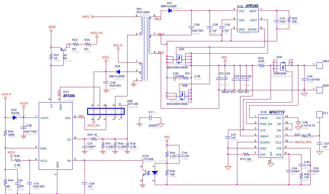
Figure 4: 140W ACF+GaN PD3.0 Adapter EVB Schematic – ACF Circuit
