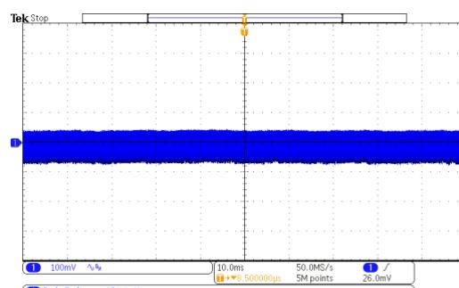
Figure 38: 264V<sub>AC</sub>/50Hz @5V/3A,  $\Delta V=121.4\text{mV}$
