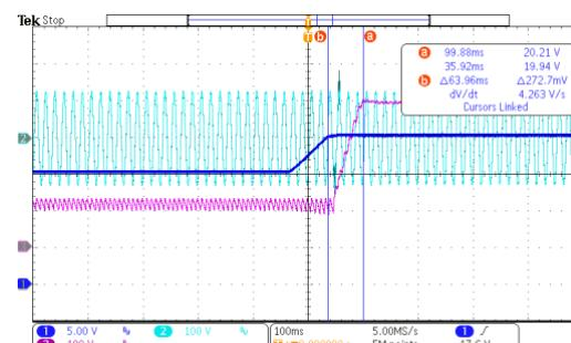
CH1:VBUS, CH2:AC Input, CH3:VPFC
