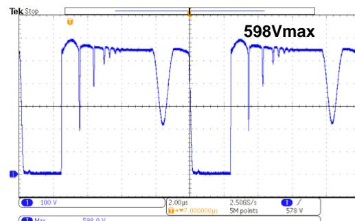
Figure 30: 20V/7A @264V<sub>AC</sub>/50Hz
