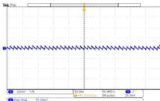
Figure 43: 90V<sub>AC</sub>/60Hz @15V/0A,  $\Delta V=55.00\text{mV}$
