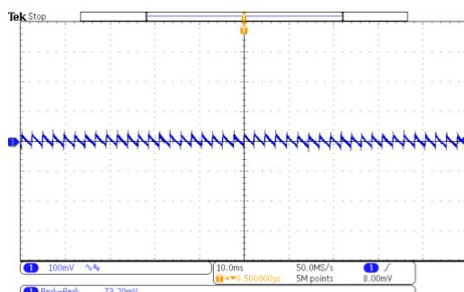
Figure 47: 90V<sub>AC</sub>/60Hz @20V/0A,  $\Delta V=73.2\text{mV}$
