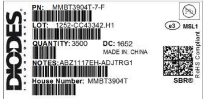
Fig. 3 Standard Label for SBR® Product that has Lead-Free Finish and is RoHS Compliant with Tin terminal finish, Moisture Sensitivity Level 1.
