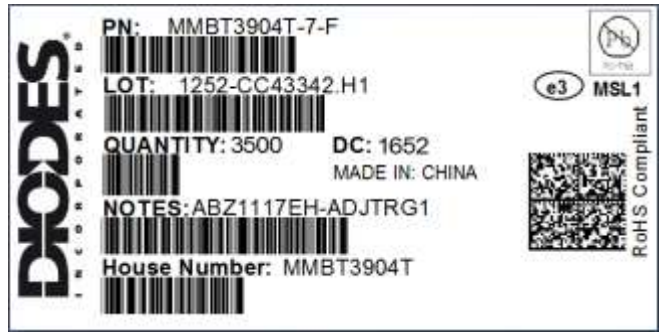
Fig. 5 Standard Label for a totally Lead-Free product, RoHS Compliant Product with Tin terminal finish and Moisture Sensitivity Level 1.
