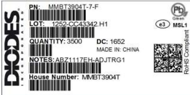
Fig. 2 Standard Label for a “Green” and Lead-Free Finish, RoHS compliant with Tin terminal finish and Moisture Sensitivity Level 1.
