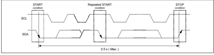
Figure 2. Starting and Stopping on I<sup>2</sup>C Bus
