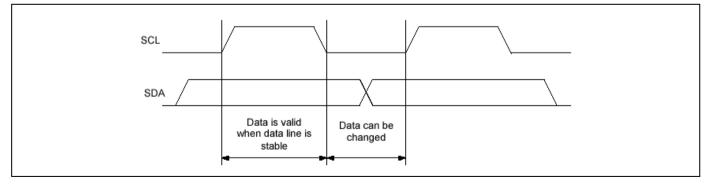
\*Note with caution that if the SDA data is changed while the SCL line is at high level, it is treated as a START, RESTART, or STOP condition.
