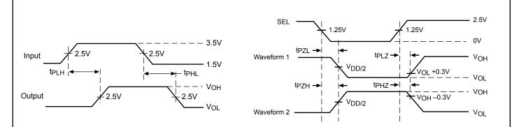
**Voltage Waveforms Propagation Delay Times**
