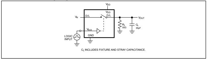
Figure 1. AC Test Circuit
