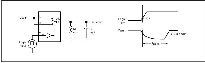
Figure 3. Break Before Make Interval Timing
