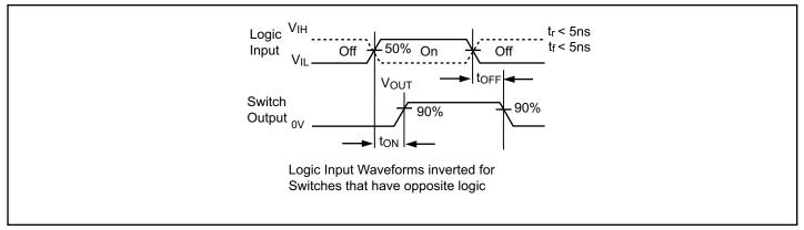
Figure 2. AC Waveforms
