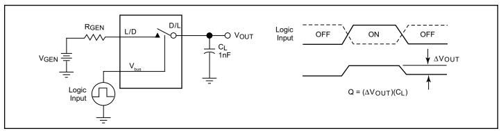
**Figure 4. Charge Injection Test**
