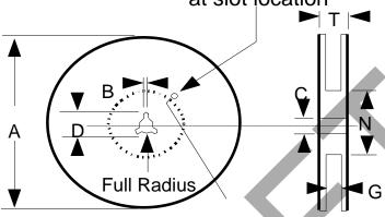
Tape slot in core for tape start 2.5(0.098)Min. width. 10(0.394)Min.depth.
