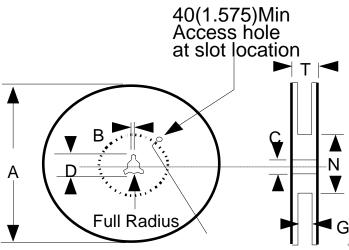
Tape slot in core for tape start 2.5(0.098)Min. width. 10(0.394)Min.depth.
