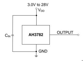
Note: 4. C<sub>IN</sub> is for power stabilization and to strengthen the noise immunity, the recommended capacitance is 10nF to 100nF. R<sub>L</sub> is the pullup resistor.
