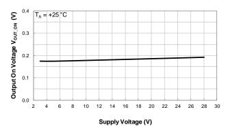
Output On Voltage vs Supply Voltage
