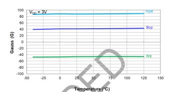
Switch Points Bop and Brp vs Temperature
