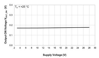
Output ON Voltage vs Supply Voltage
