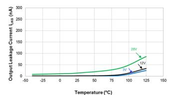
Output Leakage Current vs Temperature
