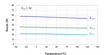
Switch Points  $\mathbf{B}_{\text{OPS}}$  and  $\mathbf{B}_{\text{RPS}}$  vs Temperature
