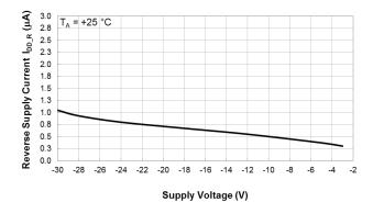
Reverse Supply Current vs Supply Voltage
