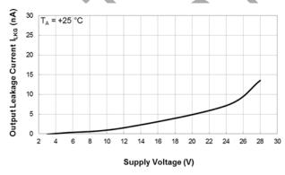
Output Leakage Current vs Supply Voltage
