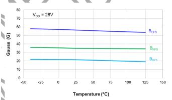
Switch Points  $\mathbf{B}_{\text{OPS}}$  and  $\mathbf{B}_{\text{RPS}}$  vs Temperature
