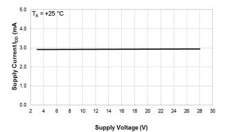
Supply Current vs Supply Voltage
