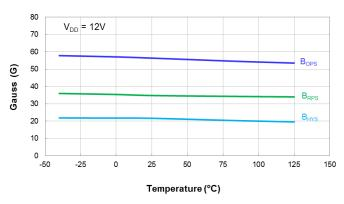
Switch Points  $\mathbf{B}_{\text{OPS}}$  and  $\mathbf{B}_{\text{RPS}}$  vs Temperature
