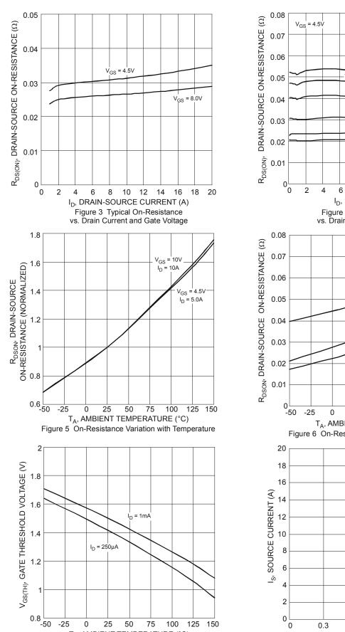
Figure 7 Gate Threshold Variation vs. Ambient Temperature
