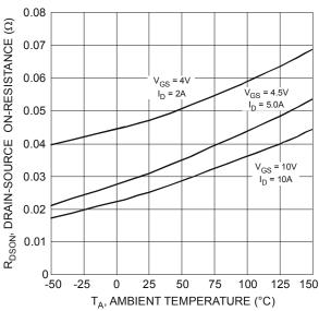
Figure 6 On-Resistance Variation with Temperature
