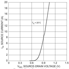
Figure 8 Diode Forward Voltage vs. Current
