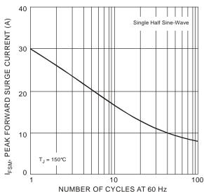
Fig.5 Max Non-Repetitive Peak Forward Surge Current
