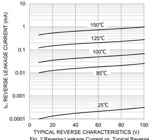
Fig. 2 Reverse Leakage Current vs. Typical Reverse
