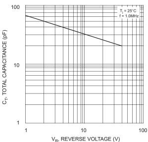
Fig. 4 Typical Total Capacitance, per element
