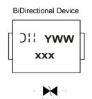
xx = Product Type Marking Code (See Electrical Characteristics Table) D!! = Manufacturers' Code Marking YWW = Date Code Marking Y = Last Digit of Year (ex: 1 for 2021) WW = Week Code (01 to 53)
