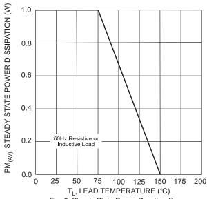
Fig. 6 Steady State Power Derating Curve
