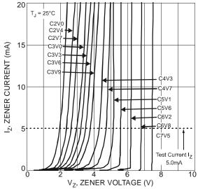
Fig. 2 Typical Zener Breakdown Characteristics
