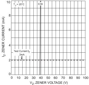
Fig. 4 Typical Zener Breakdown Characteristics
