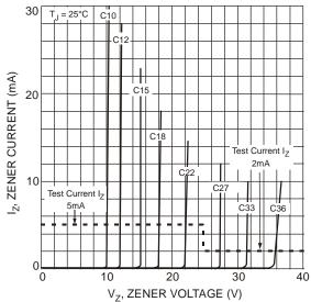
Fig. 3 Typical Zener Breakdown Characteristics
