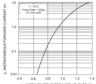
$\rm V_F$ , INSTANTANEOUS FORWARD VOLTAGE (V) Fig. 2 Typical Forward Characteristics (per element)
