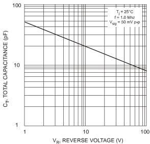
Fig. 4 Typical Total Capacitance (per element)
