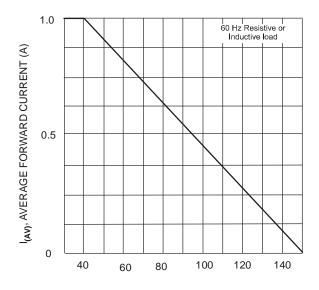
T<sub>A</sub>, AMBIENT TEMPERATURE (°C) Fig. 1 Output Current Derating Curve
