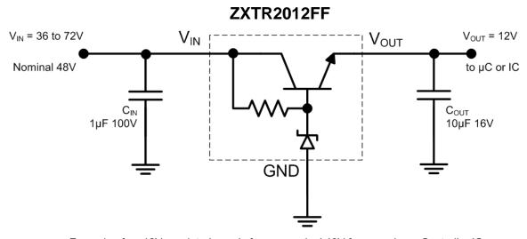
Example of an 12V regulated supply from a nominal 48V for powering a Controller IC.
