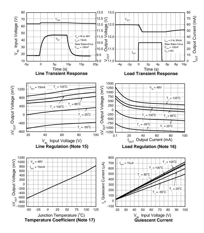
Notes: 15. Line regulation  $\Delta V_{OUT} = V_{OUT} - V_{OUT}$  (@  $V_{IN} = 15V$ ,  $I_{OUT} = 15mA$ ,  $T_J = +25^{\circ}C$ ).
