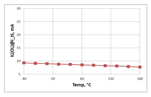
Figure 31. Open Load Detection ON State Threshold  $I_{L(OL)} = f(T_J; V_S)$
