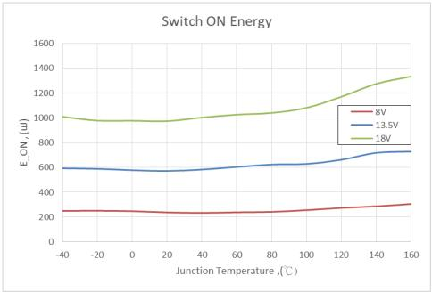
Figure 26. Switch ON Energy  $E_{ON} = f(T_J; V_S), R_L = 4\Omega$
