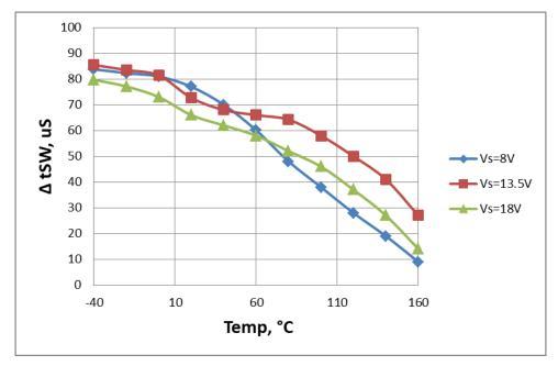
Figure 25. Turn ON / OFF matching  $\Delta t_{SW}$  = f(T<sub>J</sub>; V<sub>S</sub>), R<sub>L</sub> = 4 $\Omega$
