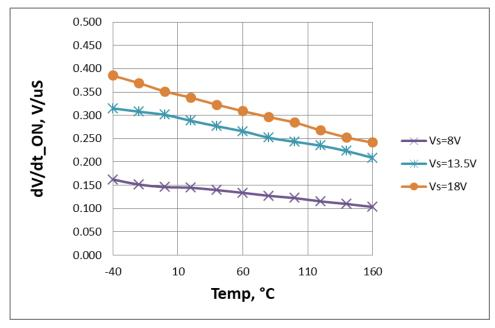
Figure 21. Slew Rate at Turn ON dV/dt<sub>ON</sub> =  $f(T_J; V_S)$ ,  $R_L = 4\Omega$
