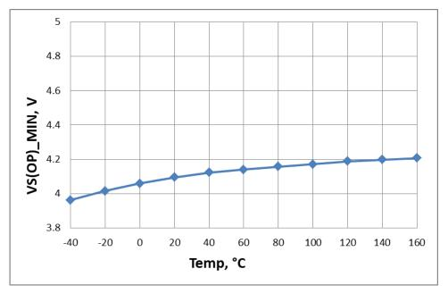
Figure 16. Minimum Function Supply Voltage  $V_{S(OP)\_min} = f(T_J)$
