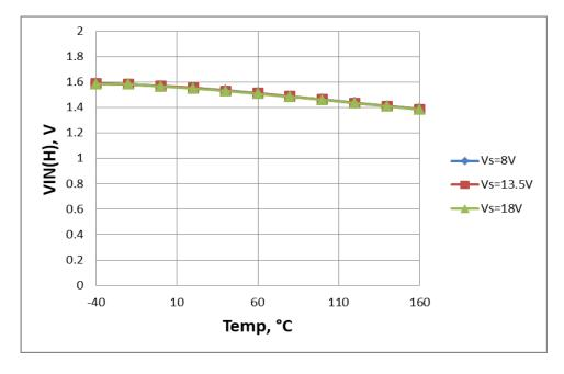
Input Voltage Threshold OFF to ON
