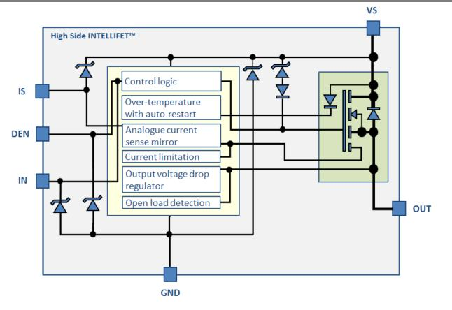
Figure 2. Functional Block Diagram of ZXMS81045SP
