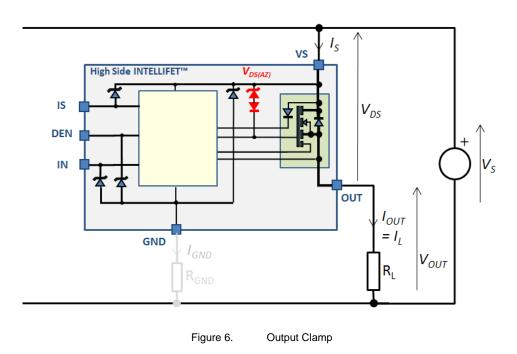
A low-impedance active voltage clamp uses the MOSFET channel to limit the maximum voltage across the MOSFET drain-source terminals, limiting the swing of OUT below Vs to safe  $V_{DS(AZ)}$ . This prevents avalanche of the MOSFET or associated circuitry.
