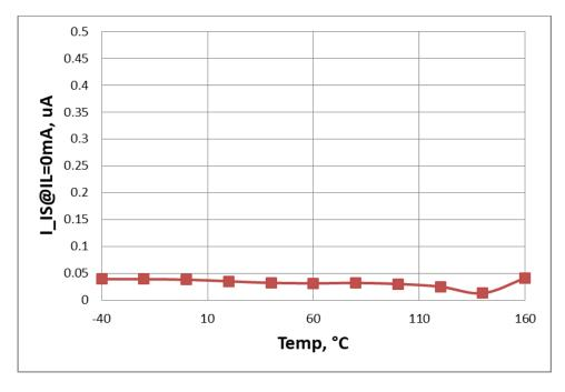
Figure 30. Current Sense at no Load  $I_{IS} = f(T_J; V_S)$
