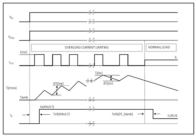
Figure 12. Overload Protection Diagram
