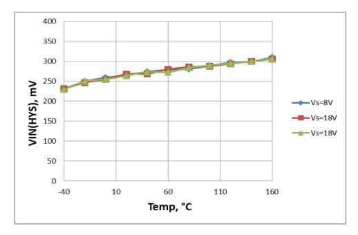
Figure 36. Input Voltage Hysteresis  $V_{IN(HYS)} = f(T_J; V_S)$
