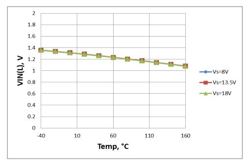
Figure 34. Input Voltage Threshold  $V_{IN(L)} = f(T_J; V_S)$
