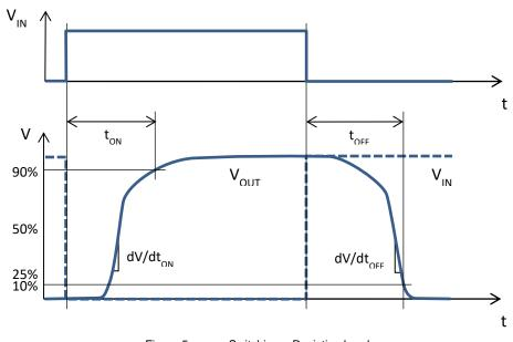
Figure 5. Switching a Resistive Load
