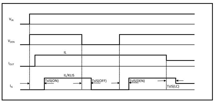
Figure 13. IS Signal Timing Diagram
