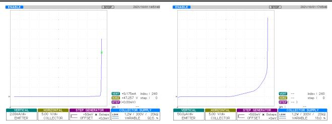
Figure 7. Typical V<sub>DS</sub> Clamp Characteristic
