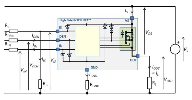
Figure 1. Typical Application Configuration
