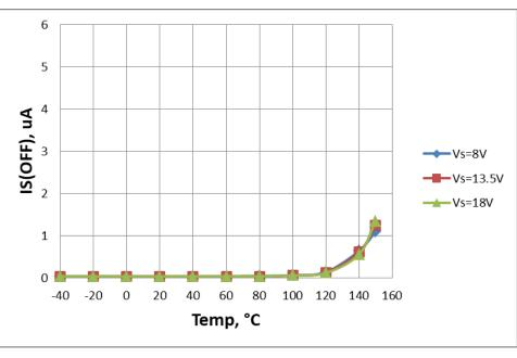
Figure 19. Standby Current for Whole Device with Load.  $I_{S(OFF)} = f(T_J; V_S)$
