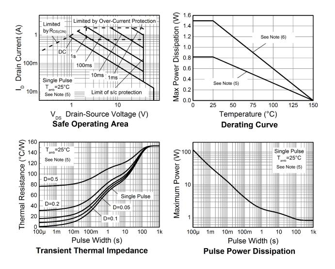
Notes: 5. For a device surface mounted on 15mm x 15mm single sided 1oz weight copper on 1.6mm FR-4 board, in still air conditions. 6. For a device surface mounted on 50mm x 50mm single sided 2oz weight copper on 1.6mm FR-4 board, in still air conditions.
